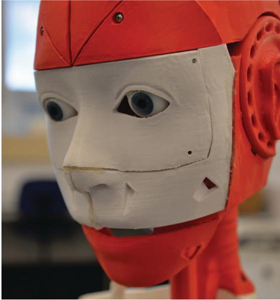
Fig. 5. 3D printed head of an Inmoov - an open-source project for a humanoid robot, selected and built by students at the club.
